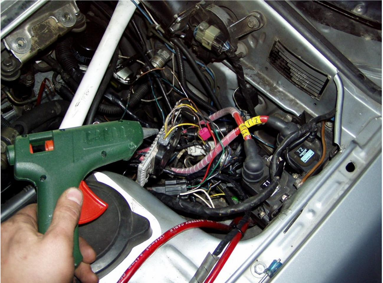
After you've done, check the wiring! When you've done, check the wiring again! Always solder the wires and use shrink tube and tape, lots of tape!
